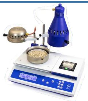
Almost 70 years of experience with modern technology forms the basis for the ULTRA X moisture analyser. Precision weighing technology, simple operation, good functionality and design and a robust structure are combined in a practice-oriented manner.
