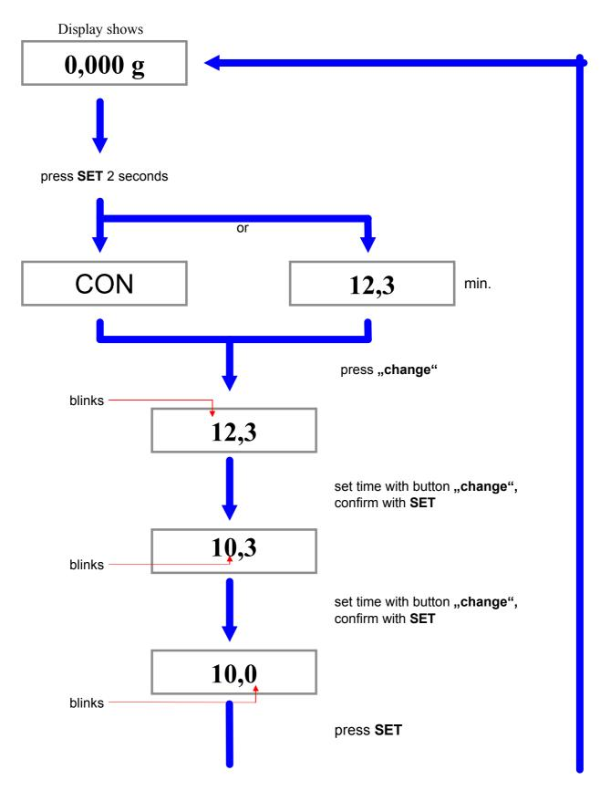
Timer set to 00,0 sets the instruments into the automatic mode.
